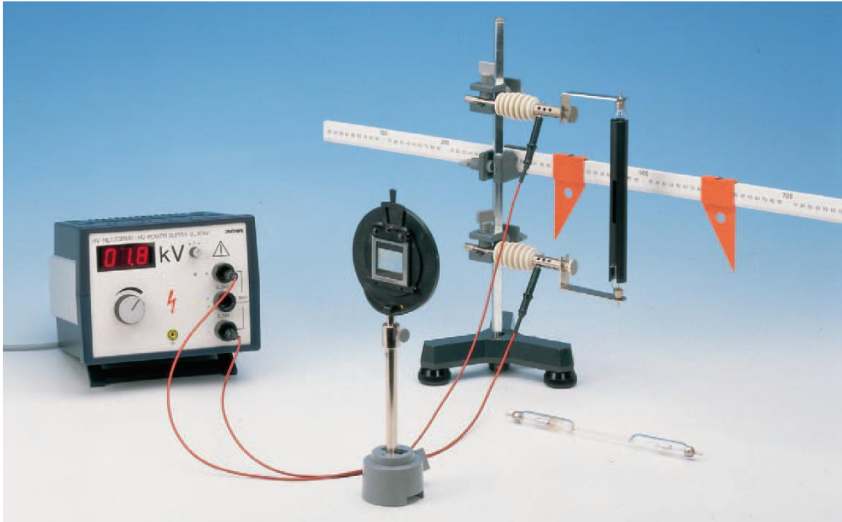
Fig.1: Experimental set-up for measuring the spectra of He and Hg.
