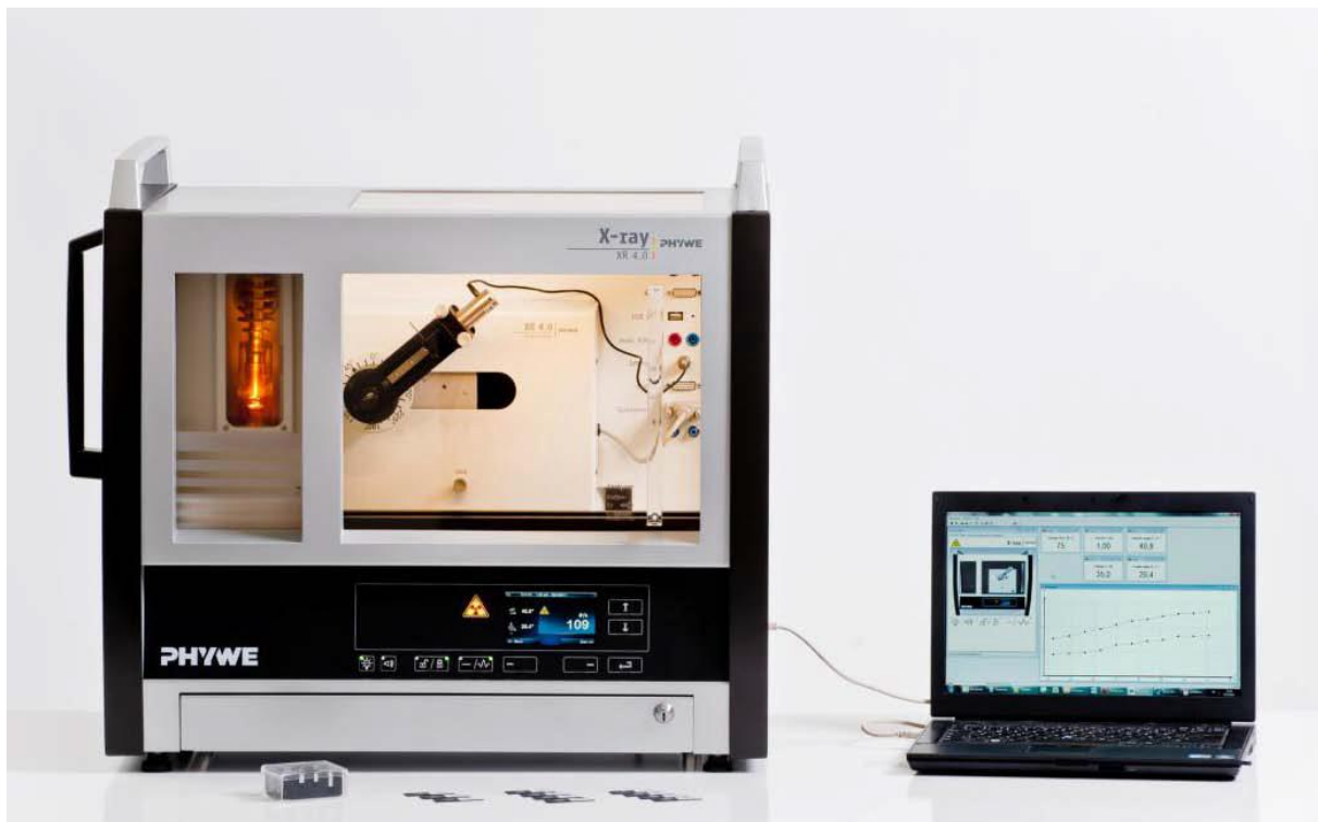
Fig.1: Experimental set-up for determining linear absorption coefficient of Al and Zn.
