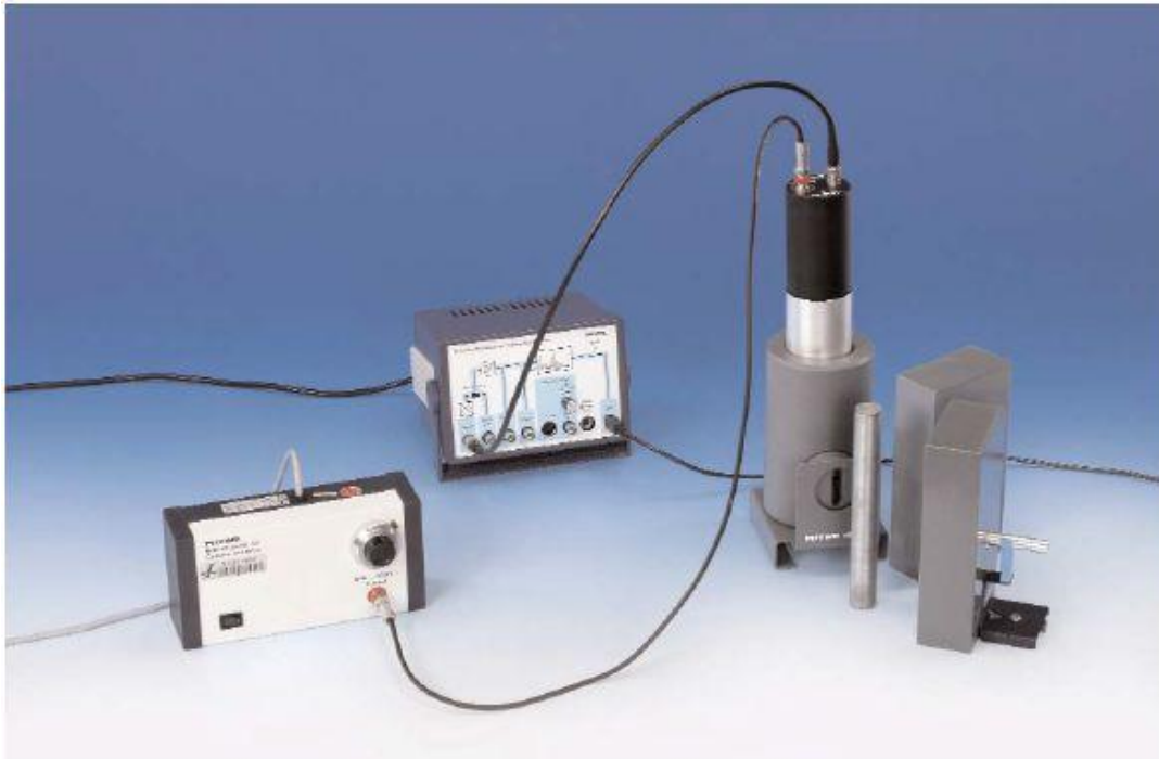
Fig.2: Experimental set-up for Compton effect.
